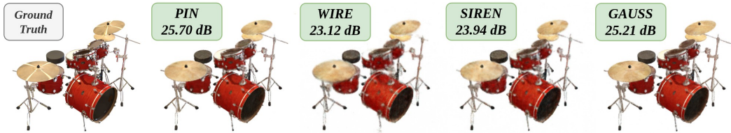
Figure 6: Novel View Synthesis Capabilities of PIN: PIN achieves the highest PSNR in novel views performance as compared to existing INRs. While existing INRs tend to produce blurry novel views in feature-dense areas, PIN’s ability to preserve maximum energy in a given state allows it to encode intricate details into its weights and biases, and produce novel views that exhibit the highest similarity to the ground truth.
